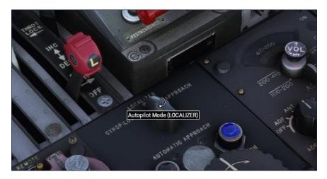
Despite the name, this is simply an autopilot mode that tracks a signal with lateral guidance, in this case the GPS steering signal. This can also be a VOR or a Localizer.
