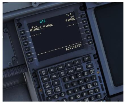
RTE Page 2 and further are where you actually enter the route information. The VIA and TO columns on the left and right sides of the screen refer back to the earlier highway analogy. The right side TO column is where you're going and the left side VIA column is how you're getting there. You can see right now that we have one line that was already filled in automatically by our SID selection – we're going to FAMUK VIA the MINNE5 SID procedure.
