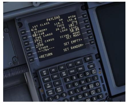
The PAYLOAD page is used to load passengers and cargo. The prompts on the right side are quick-load presets and on the left side you can type and line select the exact number of first and coach class passengers, along with the weight in the fore and aft cargo compartments.
