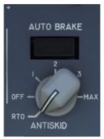
RTO stands for Rejected Take Off and will automatically apply maximum braking in the event the throttles are retarded to idle while at or above 90 knots during the takeoff roll.
