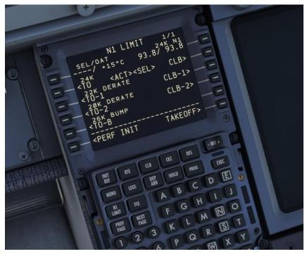
The N1 LIMIT page controls the thrust rating of the engines for takeoff and the initial climb.
