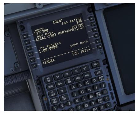
The IDENT page doesn't contain any fields for entry, but it does provide you with some valuable information such as your engine thrust rating (in this case 24,000lbs of thrust per engine), the currently installed navigation database and its valid dates, and the FMC software version, known as the Op Program.
