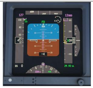
NOTE: There are conditions where LNAV will not arm on the ground. Most notably, if the first leg's course is more than 5 degrees away from the runway heading, it will not arm on the ground.
